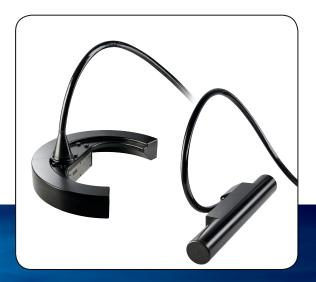
The SeaBat 7111 produces bathymetry data suitable for the generation of high resolution hydrographic charts exceeding international standards in water depths from 3 to 1000m. Operating at 100kHz, the system forms 101, 201 high-density, equi-angle or 301 equi-distant beams to cover a total receive sector of 150°.
